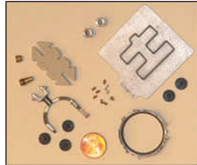
Parts with thin profiles, tabs, slots or unusual shapes present special challenges to metal finishers. Parts shown range in thickness from 0.187-0.012 inches, penny shown for scale.
